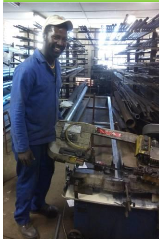
Simpfiwe Matina Works cutting metal at Albany Engineering
